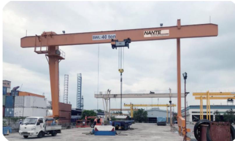
Single Girder Truss Type Gantry Crane
